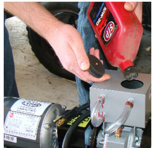
Adding oil to the oil reservoir.
